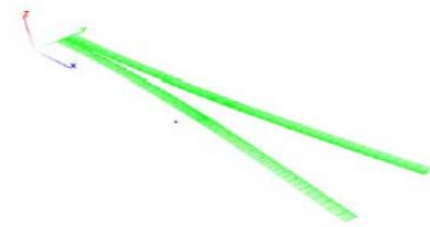
Figure 5. Crack path predicted by GENOA/PFA with Failure Criteria
