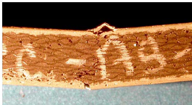
Figure 6. Failed long RCC plate specimen obtained in
